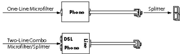
splitter. Sharing a phone outlet with two devices requires a splitter.
